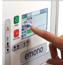
From the display all the functions and options of the device are set, and values, trends, and alarms are shown.
